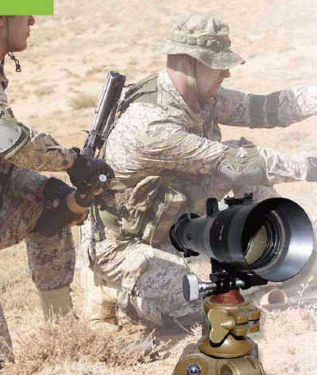
Intended for laying the gun in azimuth in the absence of natural distant aiming points and in limited visibility conditions (night, fog, fire position obscured by smoke) and can be used with MPM-44M (MON-44M) mortar sight. The collimator is provided with a level for leveling, a reticle illumination light for operation in the dark and a tripod for ease of installation. Operation temperature range is from -50 to +50° C in all weather conditions.
