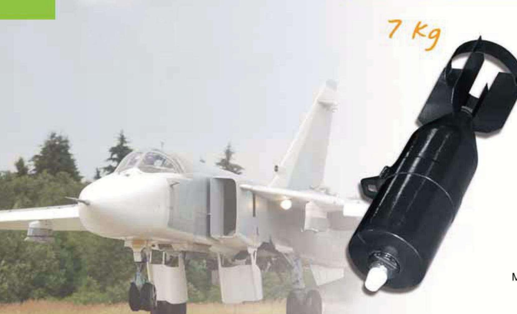
Practice aircraft bomb TAB-7 is designed for training the flight personnel bombing technique. The ammunition design ensures its practical use both in the daytime and at night. Appearing at the bomb impact a smoke cloud & a flash allow visual observation of the drop point.
