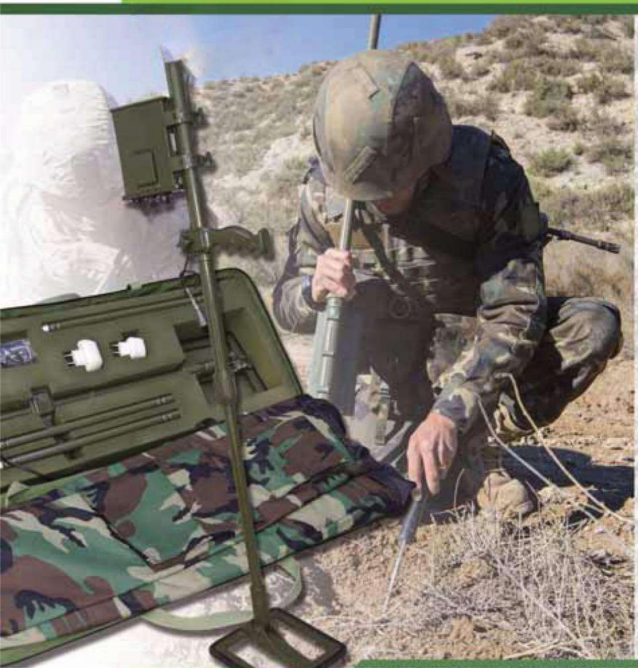
Metal Detector is designed for the searching and detection of the metal and metalic objects both underground and in water.
