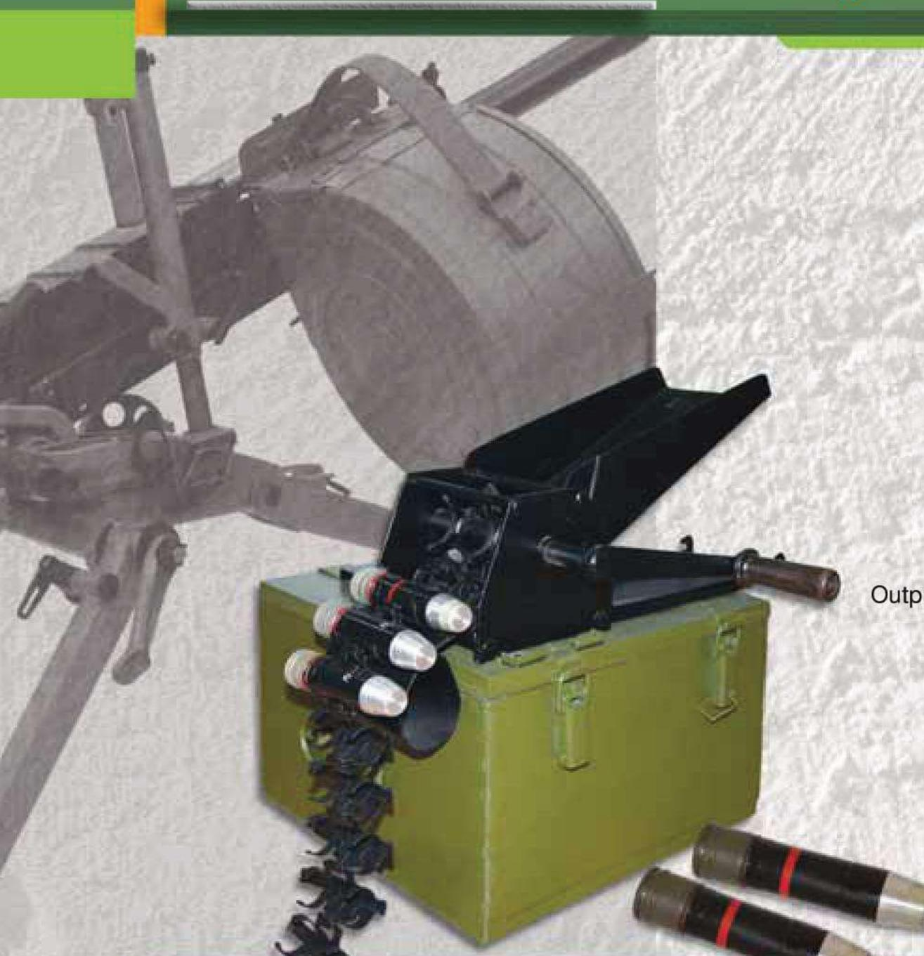
Manually operated Linking Machine is intended for linking 30x29 mm grenades for AGS-17, **AGS-30** and **ARCUS** 17AGL. The machine may be mounted on its packing or on the table.
